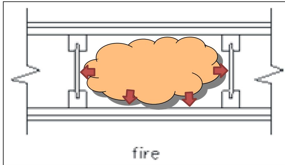
As 'fall-off' of gypsum plasterboard is related to its dehydration, simultaneous heating from both sides could influence the time until: plasterboard failure, subsequent direct exposure of the I-joist to the fire, local structural failure of the I-joist due to this direct fire exposure, and hence premature failure in terms of fire resistance of the wall or floor in question.
