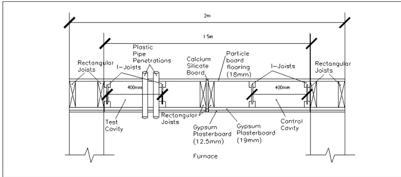
The pipe penetrations were tightly fitted within the apertures in the particle board flooring and gypsum plasterboard. The minimal annular space around the pipe penetrations remaining were then sealed with inert gypsum based plaster filler; this type of fire-stopping material being permissible in the guidance to the Building Regulations.
