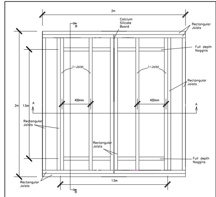
The samples contained both a 'test' cavity which was penetrated by plastic waste pipes and a 'control' cavity with no penetrations.
