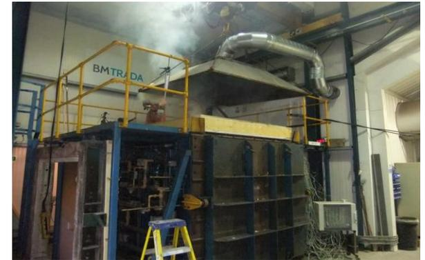
In order to examine the effect of the limitations peculiar to Scotland three reduced scale fire resistance tests were conducted on 2 m x 2 m floor samples. The discussion in this paper relates only to the first test, which would be acceptable in all of the countries of the UK as well as the Republic of Ireland.
