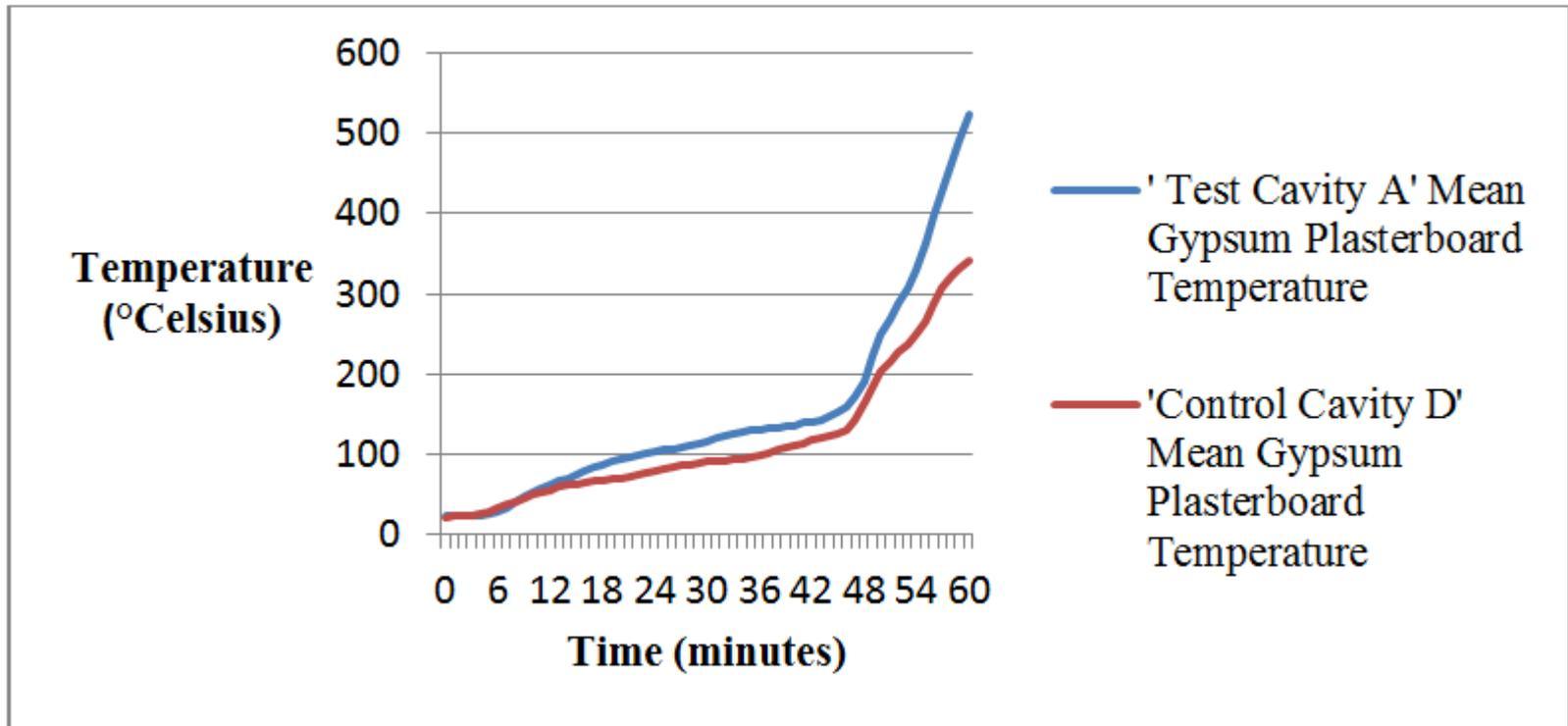
By visual observation through the furnace window, after approximately 30 minutes the first layer of 12.5 mm gypsum plasterboard had predominantly fallen off; thereafter cracks appeared in the 19 mm inner layer of gypsum plasterboard.
