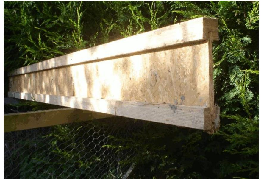
*'Manufactured timber I-joists are more efficient than solid sawn timber joists under normal temperature conditions, but may not perform as well in fire if the Webs are thin, because of strength loss due to charring of the web.'*
