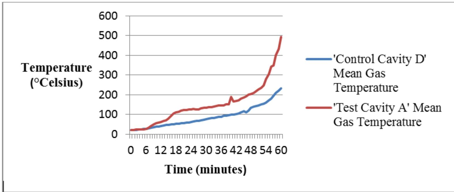
After approximately 12 minutes the test cavity's mean gypsum plasterboard temperature was consistently above that in the control cavity, suggesting that the inclusion of the pipe penetrations did lead to additional heating of the rear of the gypsum plasterboard.
