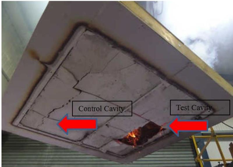
It was noted that even before the pipe penetration apertures joined and formed a single larger hole some combustion was evident in the test cavity; flames appeared sporadically through the 40 mm apertures into the furnace. This sporadic flaming combustion was probably limited by the amount of oxygen available for combustion within the cavity and by the oxygen available within the furnace.
