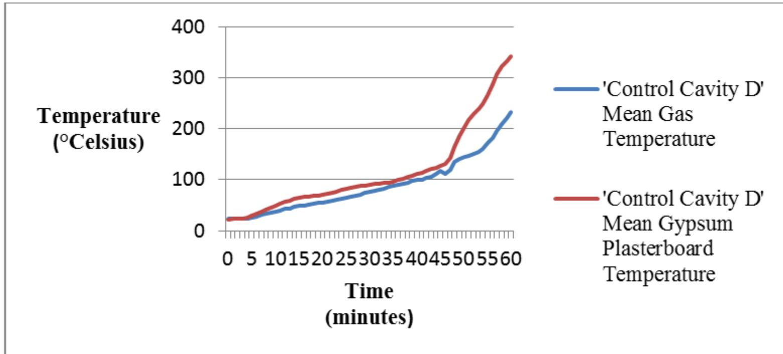
In the test cavity, for part of the test period the converse was true. This reversed towards the end of the test period when the gypsum plasterboard temperature exceeded the gas temperature, which approximates with the time that cracks between the penetration apertures joined, forming one larger hole in the inner layer of 19 mm gypsum plasterboard.
