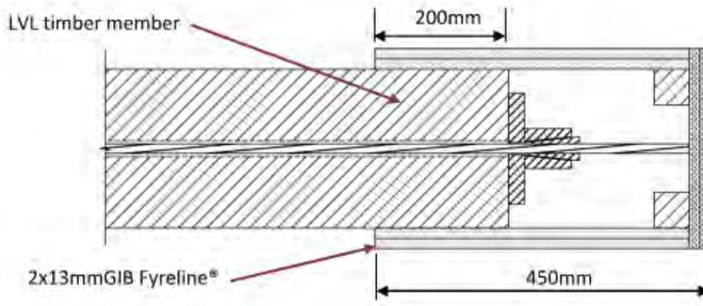
Figure 59 – Gypsum board protection for post-tensioning anchorage (Spellman, The Fire Performance of Post-Tensioned Timber Beams, 2012)
