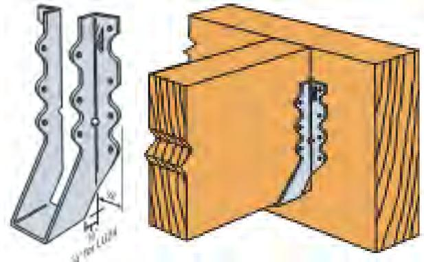
Figure 16 – Typical joist hanger framing (HomeBuildingAnswers, 2008)
