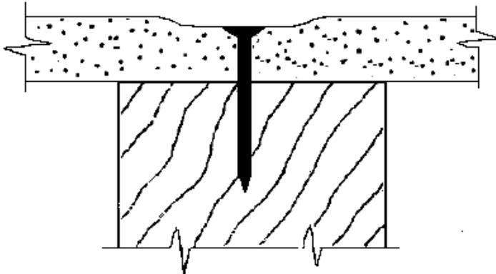
Figure 14 – Example of gypsum board framing to timber wall studs (GypsumAssociation, 2013)
