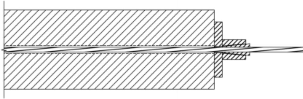
Additional benefits of post-tensioned timber buildings are that all elements can be prefabricated offsite to minimize onsite work and reduce total construction time and cost. The structure has also been shown to perform well in seismic testing (STIC, 2009).
