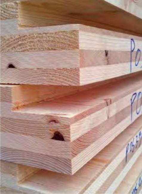
Figure 27 – CLT wall and floor elements (FPInnovations, Solid Advantages, 2012)
