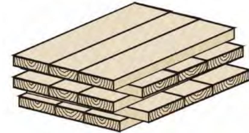
Figure 26 – 5-layer CLT panels with pre-cut notches (FPInnovations, Solid Advantages, 2012)
