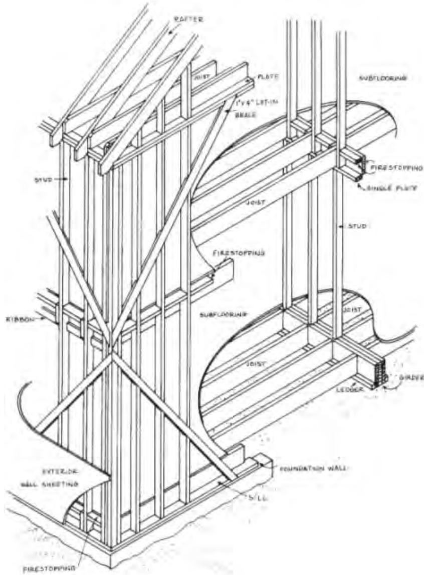
Figure 10 – Typical second floor framing showing floor joists, wall studs and plywood protection (AFPA, 2001)
